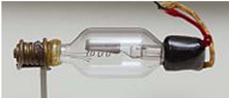
Over a hundred years development has resulted in many Triodes, large and small. The basic design has remained much the same. An evacuated container, usually glass, holds three signal connections, seen in the drawing as the Cathode, Grid and Plate (the Plate is also referred to as the Anode). In addition you see an internal heater, similar to a light bulb filament, which is used to heat the Cathode.
