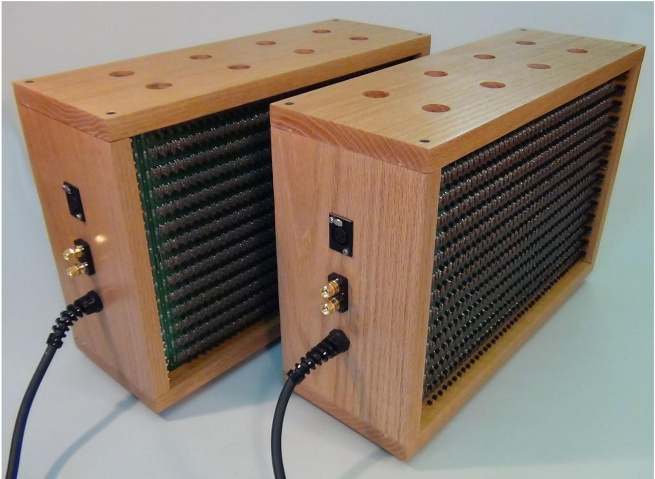
What you can't see is that there are two boards to each box, one on each side. The power supplies are external, and the input is via balanced XLR connectors.
