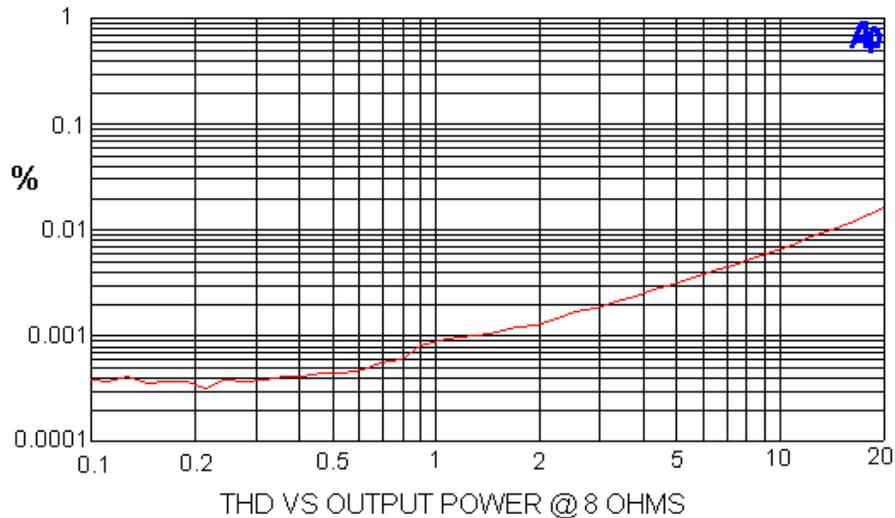
Note that the amplifier was driven by an Audio Precision System 1, whose maximum output is a little under 14 volts rms. Routinely the amplifier can do a few volts more, but that's just icing on the cake.
