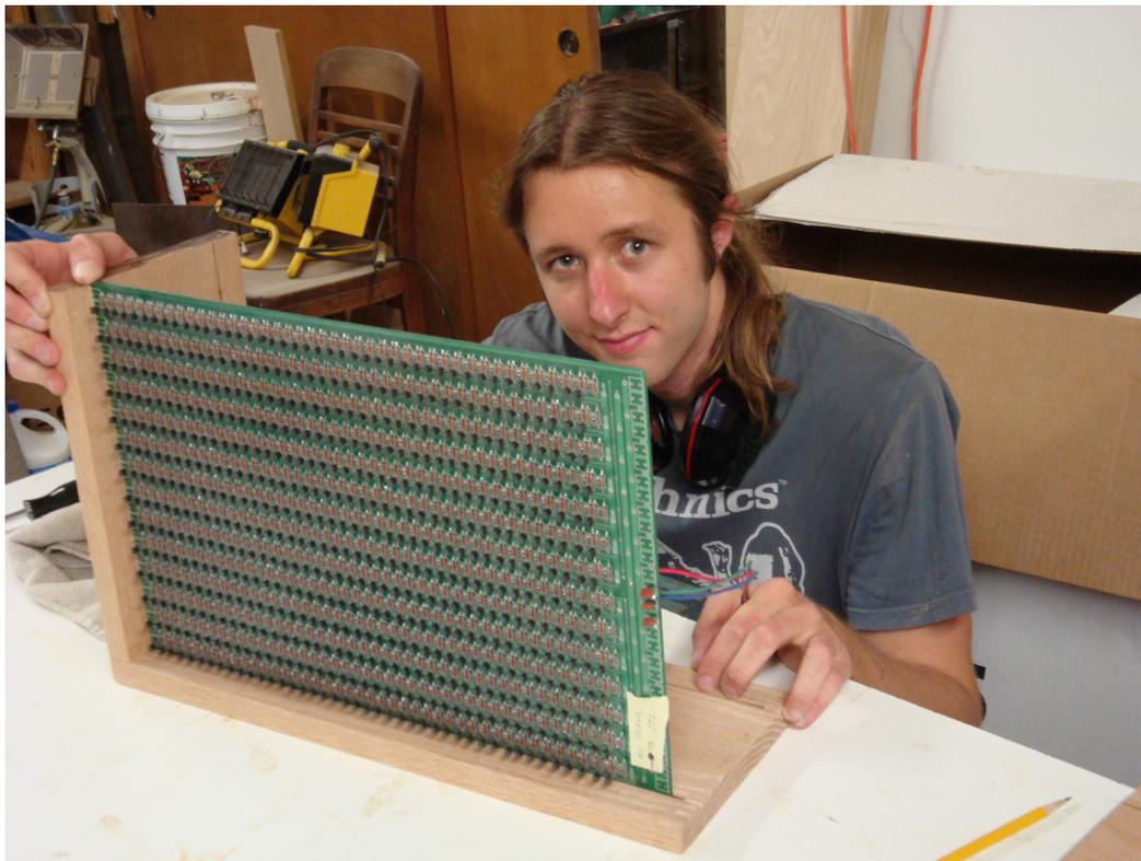
Roth tested the  $I_{DSS}$  of each Jfet and soldered them into the boards:
