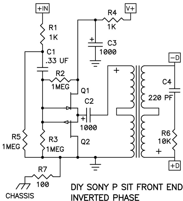
This circuit is mounted on a separate board from the output stage, and consists of a pair of complementary Jfet followers which drive the primary coil of the Edcor 600/15K step-up transformer. The Jfets are selected Toshiba 2SJ108 and 2SK370, the same chips as 2SJ74 and 2SK170 but in a smaller package, which provides for an input impedance to the amplifier of 330 Kohm and low distortion.
