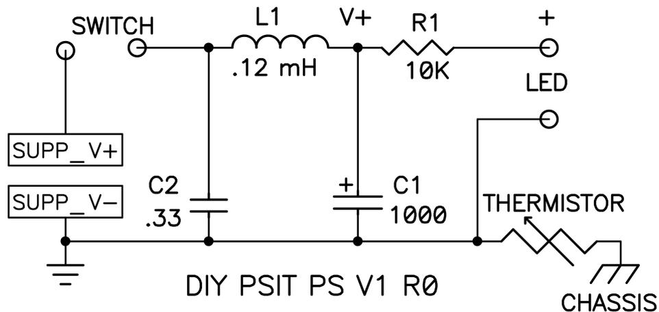
The Meanwell supply chosen was the most quiet tested, and in the prototype circuit I did not see the switching noise at the output. Nevertheless I anticipated that it might be a cause for *audio nervosa*, so I worked this simple circuit up. Now I can't see the noise on the supply rail either. Nice to note that the channels draw a literally constant DC current – no modulation of the supply.
