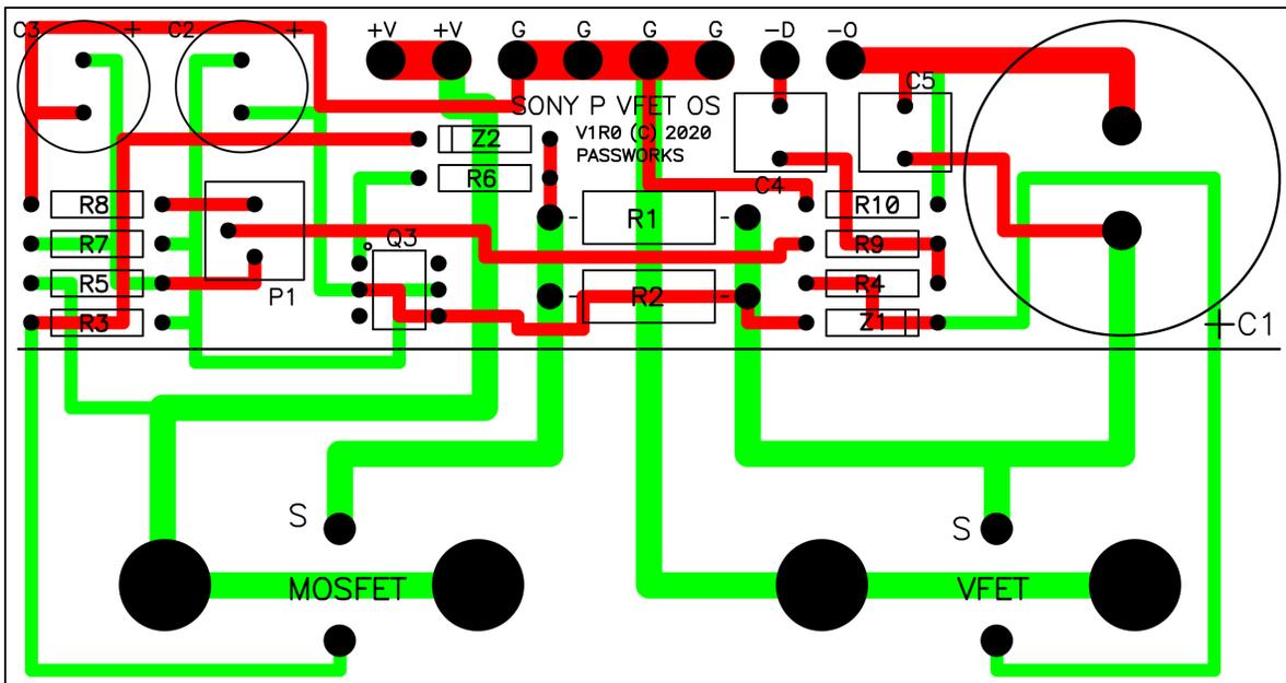
This is the pc board for the power supply filter:
