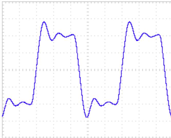
Without the transformer the response of the output stage alone is better and without resonance. This is dependent on the source impedance, so your mileage may vary:
