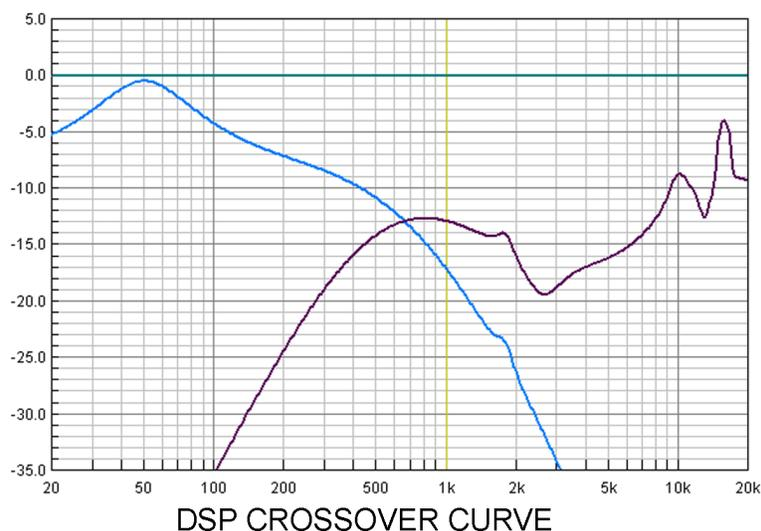
It's got lots of little bumps, peaks and dips, each correcting for the curve that Siegfried obtained when he put a microphone in front of the speaker and measured the response.
