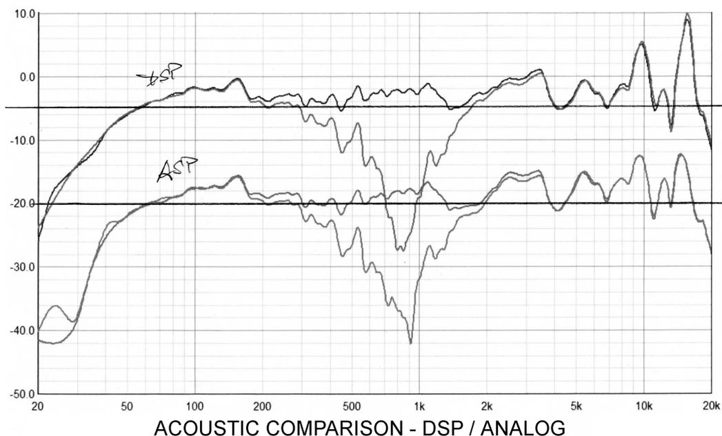
We speculated a bit on why that might be. One possibility was that the anomalies of the high end driver might vary from unit to unit. The other was that at wavelengths of less than an inch, variation of microphone position might account for it.
