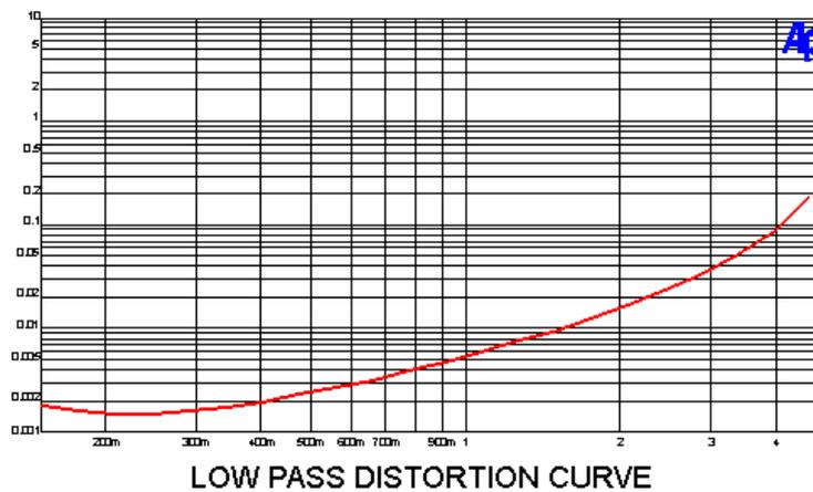
Here is the distortion of the mid/hi filters at 900 Hz:
