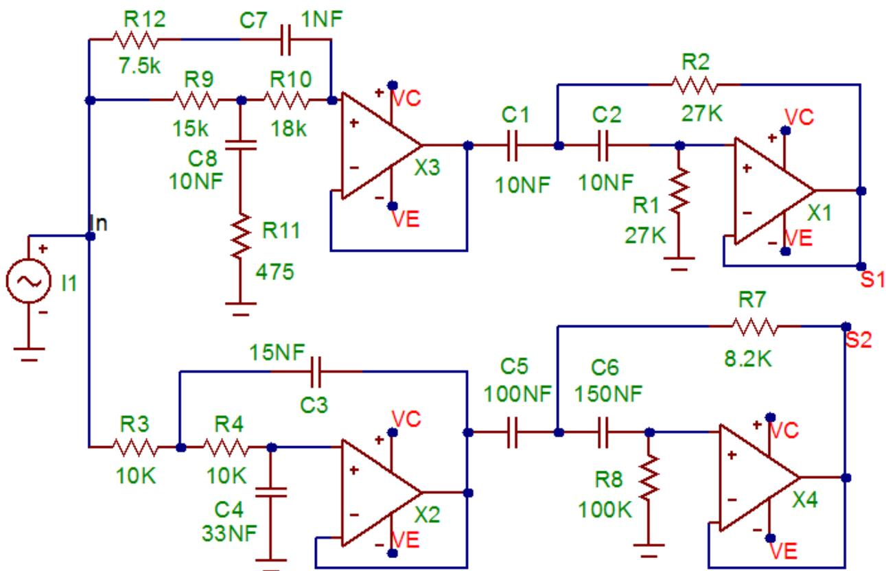
Interestingly, the filter topology is remarkably close the First Watt B5 crossover, which caters to full range drivers and woofers in open baffle enclosures.
